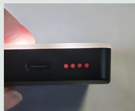
Power on to check battery life, which will be indicated on the side with the charging port. 4 lights is full charge, 2 is 50% etc...
